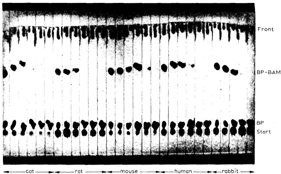
Fig. 2. TLC negative picture of the time course of the hydrolysis of BP-BAM by serum specimens from different species.
